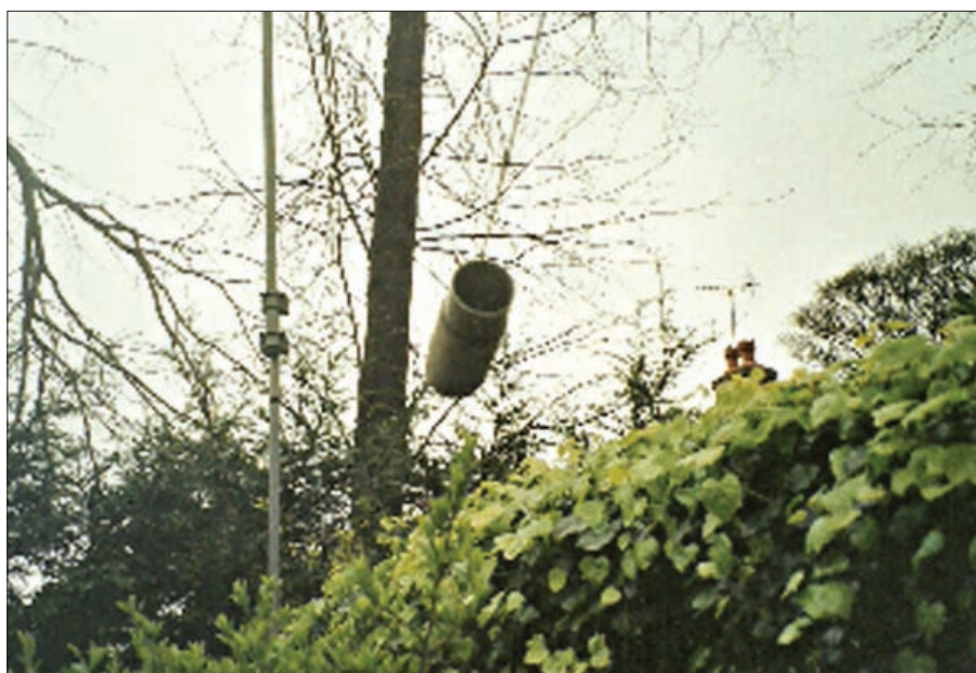
Fig. 4: The loading coil, L1 consists of 30 turns of antenna wire wound on a 50.8mm (2in) former and is placed 9.145m from the 'top' of the shunt coil. The outer end of the antenna has its length trimmed to give resonance of the whole system. As it might vary between about 9 and 12m a little experimentation will be needed. Some form of weather protection will probably be needed.
