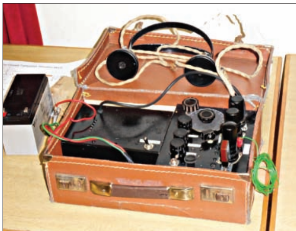
Fig. 1: Alan Stepney G8BLW's winning entry – a modern replica of the Second World War Paraset. Judge and sponsor of Geoff's Challenge' – Geoff Fowle M0CJC told the audience that Alan had "produced a replica that was the nearest to the real thing".
