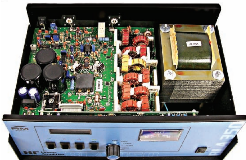
Fig. 3: There's one main printed circuit board (p.c.b.) housing the two m.o.s.f.e.t.s and a very large heat sink underneath.
