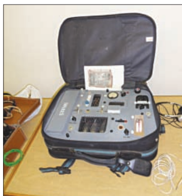
Fig. 2: Colin Davis G0JII's replica Paraset even had valves with heaters that illuminate! – It is a cleverly disguised modern MFJ Cub h.f. c.w. transceiver for 14MHz, built into a modern suitcase.
