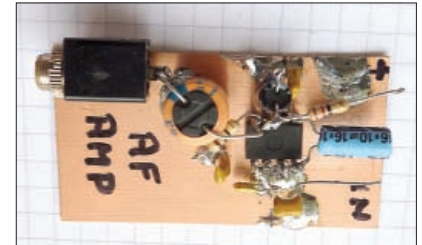
Fig. 2: (a) Illustrating the 'dead bug' style of construction. (b) contrast the stylised layout with the picture shown here.
